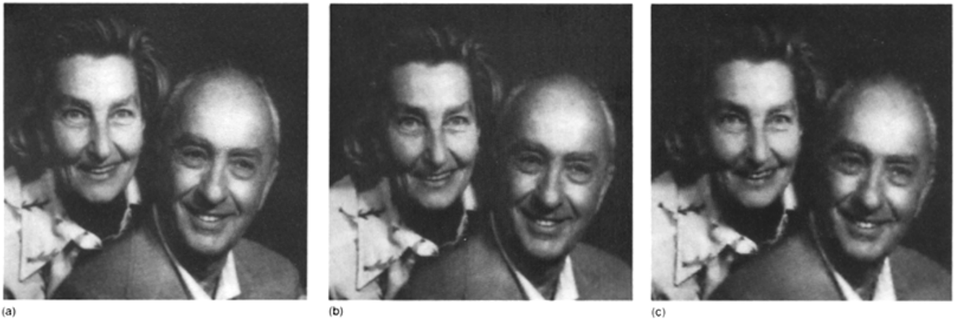
Fig. 5. Pyramid data compression. The original image represented at 8 bits per pixel is shown in (a). The node values of the Laplacian pyramid representation of this image were quantized to obtain effective data rates of 1 b/p and 1/2 b/p. Reconstructed images (b) and (c) show relatively little degradation.
