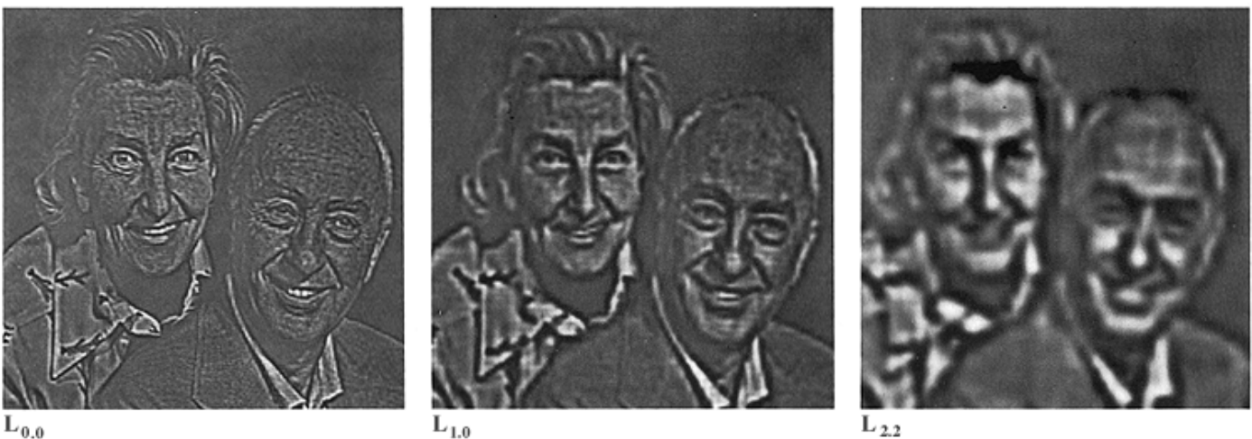
Fig. 4b. Levels of the Laplacian pyramid expanded to the size of the original image. Note that edge and bar features are enhanced and segregated by size.
