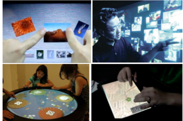
Figure 1: The majority of current MT applications regard actions such as drag, resize and rotate of photos: a) Microsoft Surface Collage application, b) Jeff Han manipulating pictures with two finger gestures [3], c) multiplayer MT demo on PyMT[4], d) MT navigation application[4].
