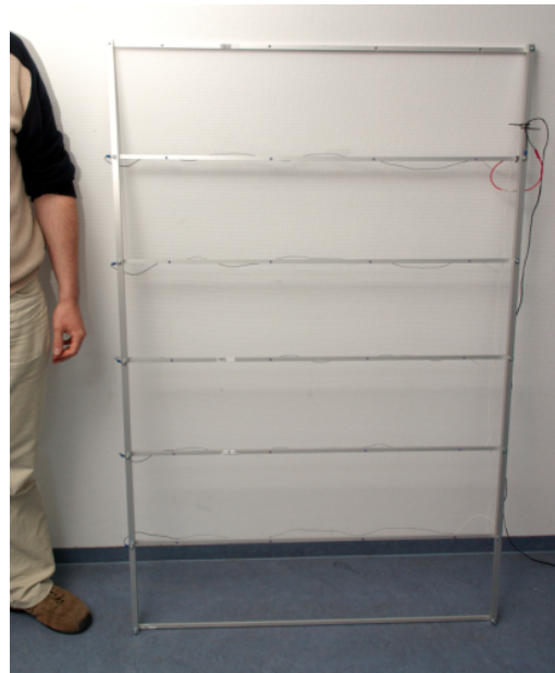
Figure 7. LED mounting grid
