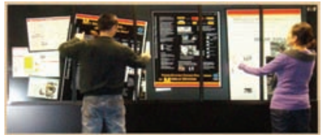
Figure 1. Our multi-touch wall is 3025mm × 1052mm with a resolution of 9600 × 1080 pixels, and capable of detecting multiple points of contact simultaneously.
