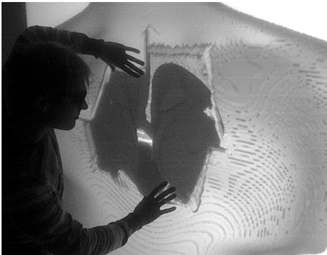
Figure 2: A user deforms a medical volume dataset using an iMUTS based on FTIR and passive back projection.
