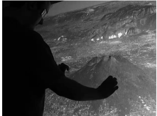
Figure 1: User interacting with iMUTS in a landscape planning scenario where depth cues are important, e.g., in a landslide risk management scenario. Geospatial data is displayed in anaglyph mode.
