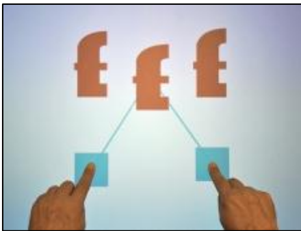
Figure 15. A user achieves higher precision 2D translation by holding one proxy and moving the other.
