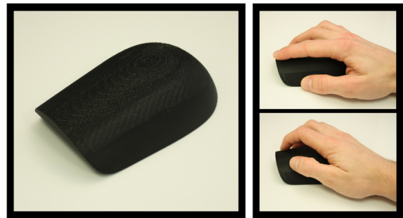
Figure 8. Cap Mouse employs a matrix of capacitive touch-sensing electrodes to track the position of the user’s fingertips over its surface.
